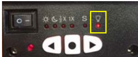
Figure 22 Polar scope LED intensity adjustment
