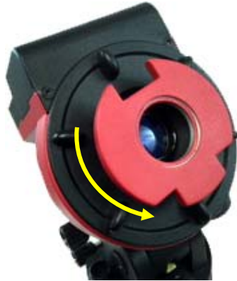
Figure 21. Adjust polar scope position if needed
